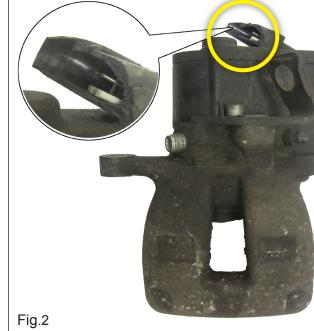
Cracked plug connector (Fig.2)
