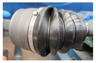
The new design of the wheel-side CV-Joint boot allows the boot to keep its characteristics even with the highest steering angles, leading to a reduced stress and longer life for the boot itself.
