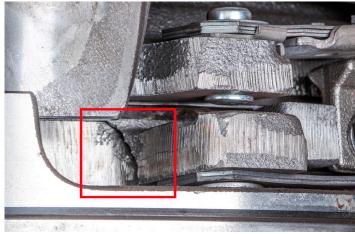
Image 1: Cam break at the fixture of the tangential leaf spring
