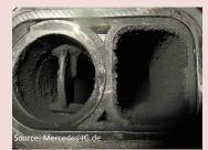
The issue of unclean combustion in engines is a continuous nuisance in garages everywhere – and the cause of many apparent failures of parts.
